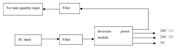
Fig 3-3 Schematic diagram of power supply module
