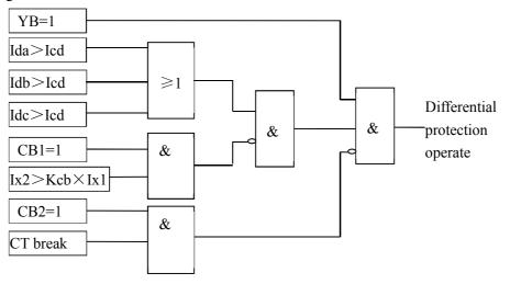
Fig. 2 Logic Diagram for Differential Protection
