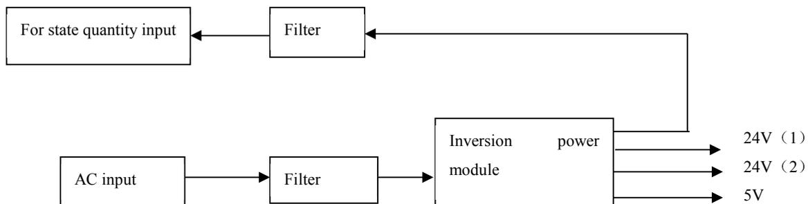
**Fig 3-3 Schematic diagram of power supply module**
