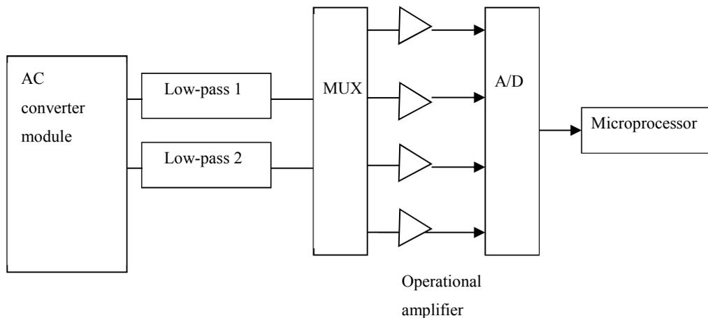
**Fig 3-2 Schematic diagram of A / D system**
