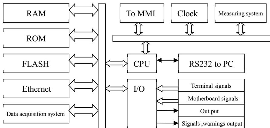
**Fig 3-1 Schematic diagram of the CPU module**
